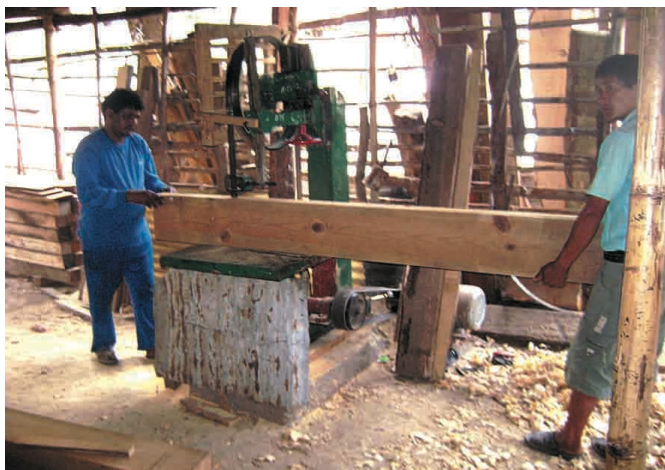
Figure 29 Saw Mill with the help of 22KW micro hydro at the town (Source: (Alternative Energy Promotion Centre, 2011)
