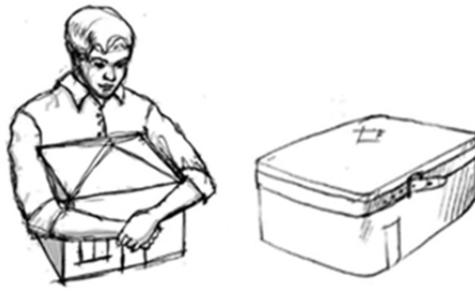
Figure 10-5 A seismic band acts like a belt (adapted from: GOM 1994)
