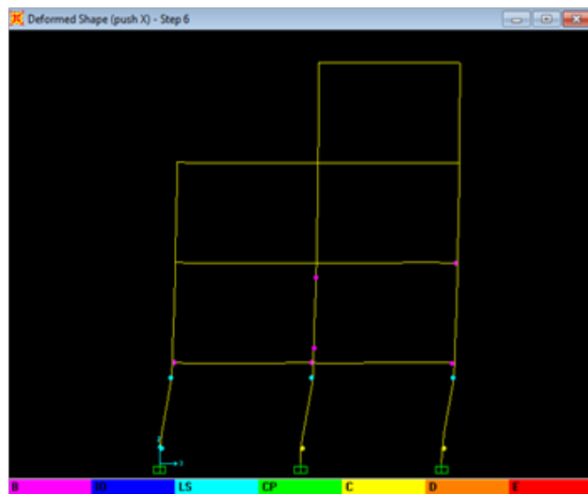
Plastic hinge (push X) of Grid 3-3
