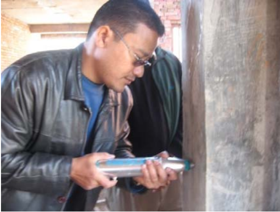
Fig 1. (a) Use of Rebound Hammer
