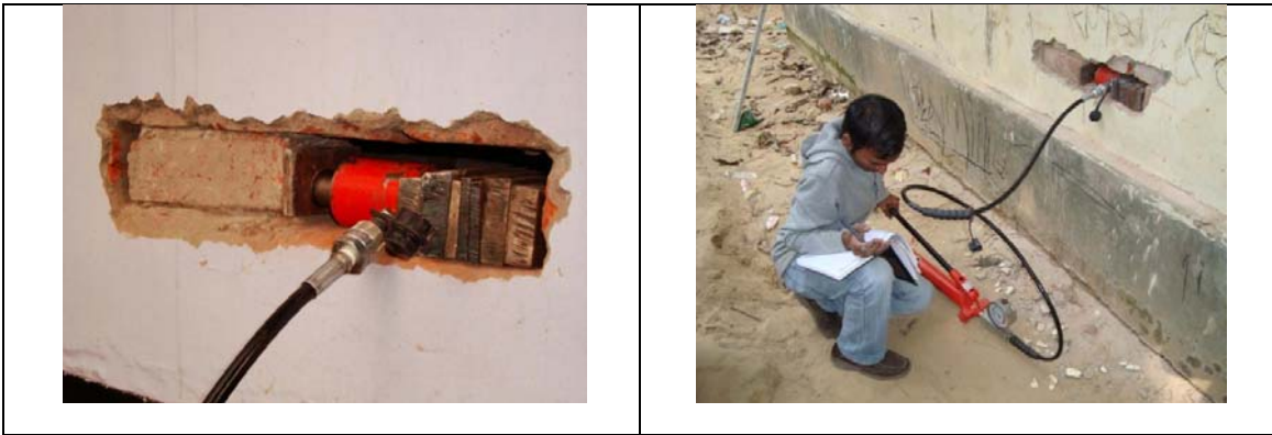
Photo 29-30: Test set up for In-situ Shear test
