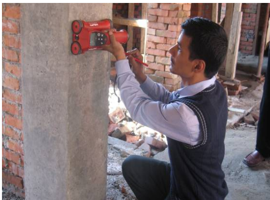
Fig 2. (a) Use of Rebar Detector for Verification of Reinforcement Details
