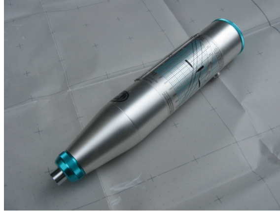
Fig 1. (b) Rebound Hammer
