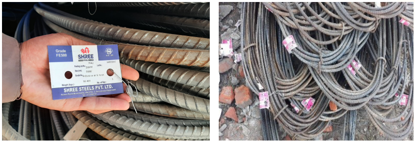
Figure 9: - Tags of reinforcement with NS standard, weight, and size
