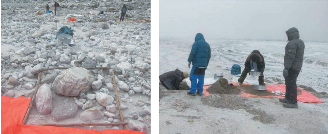
Bed sediment sampling in plots (left) and at Bhemathan (right) (photos by Clean Energy Consultants Pvt. Ltd.)
