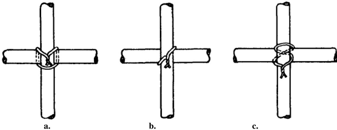
**Figure 2.2 Three methods of tying reinforcement bars**
