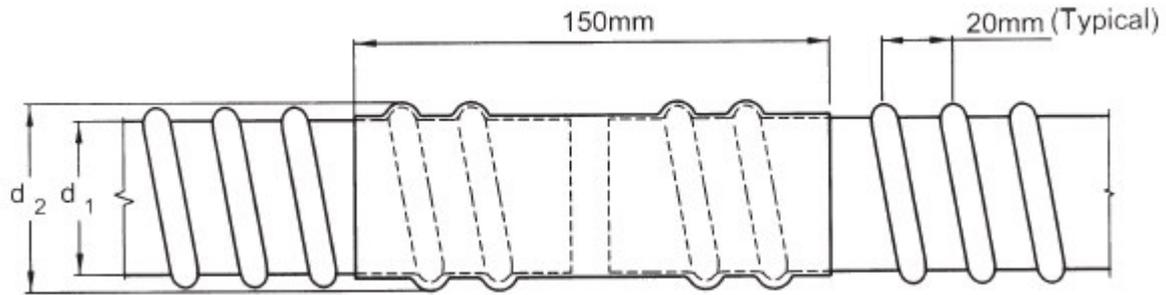
**Figure 1.5 Typical details of a sleeve coupler**
