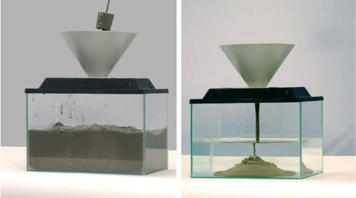
**Figure 1.1 Without or With(right) Anti-washout Admixture**
