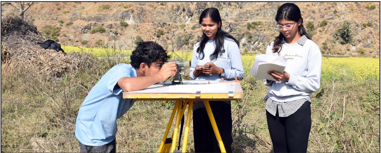
Trainees of Junior Survey Training (Fresh) Conducting Plane Table Survey at Lumsalbesi
