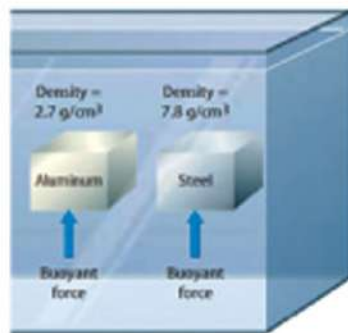
Figure 8.27 Upthrust acting on the object with the same volume
