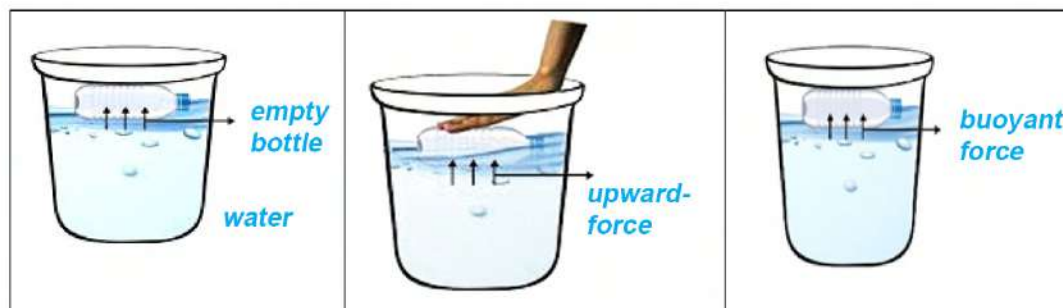
Figure 8.19 The upward force on the empty bottle when it is immersed in water
