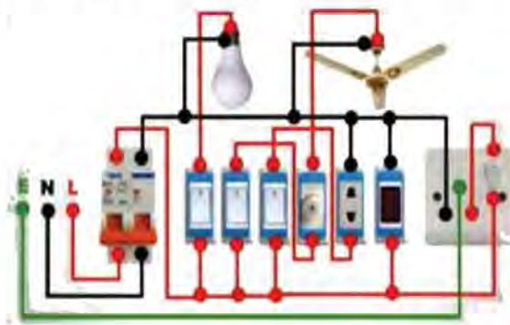
Fig 8.24 Connection of the bulbs in household electrification
