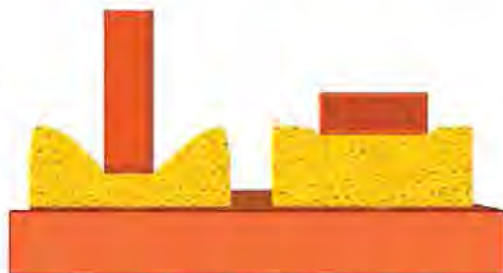
Fig 6.15 Pressure exerted by brick in different orientations.
