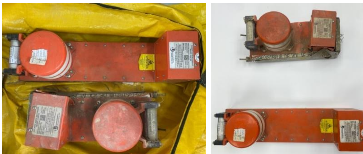
Figure 7: Condition of recorders as received by AAIC (left), and after being transported to TSIB, Singapore (right)
