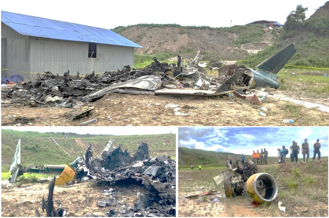
Figure 4: Top: scene at the main wreckage site, bottom: burnt fuselage and empennage sections, and the detached left engine. Images were taken on July 24 and 25, 2024.
