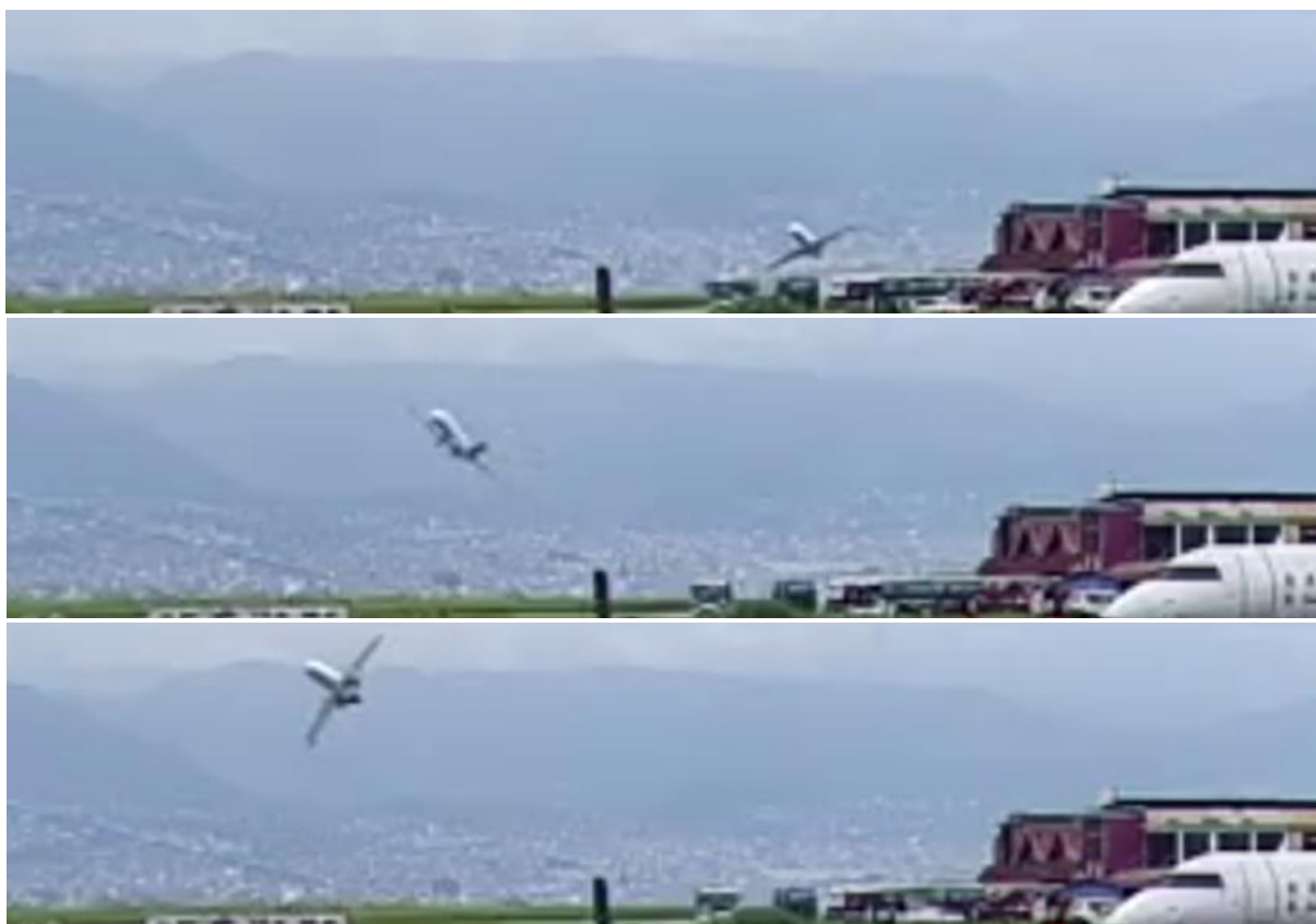
Figure 3: Event sequence with unusual attitudes leading to the accident, captured by a CCTV camera
