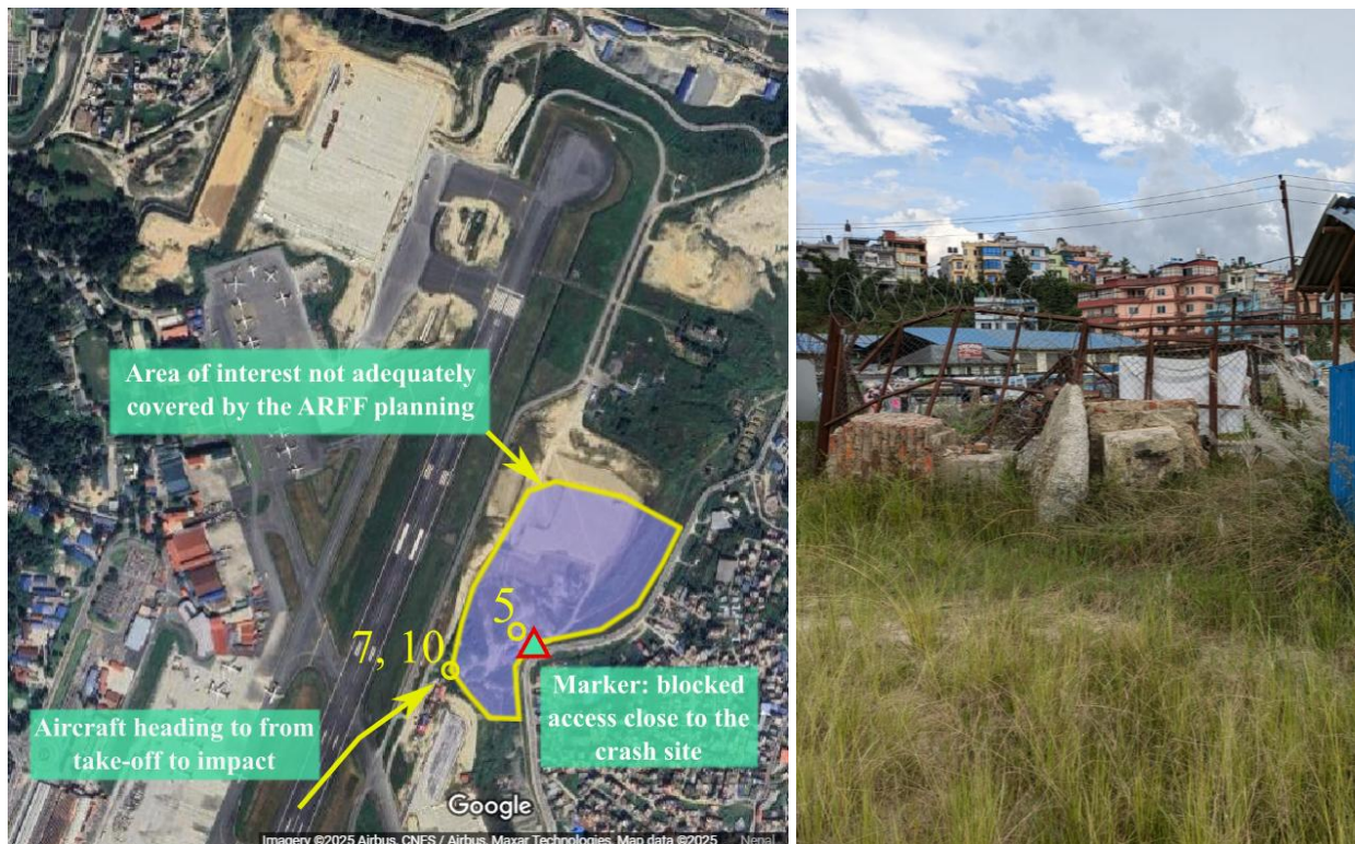
Figure 13: Blind region in the area of interest that hindered effective rescue and firefighting efforts. The markers 5, 7 and 10 are as listed in Figure 9. The blocked access marked near 5 is shown on the right.
