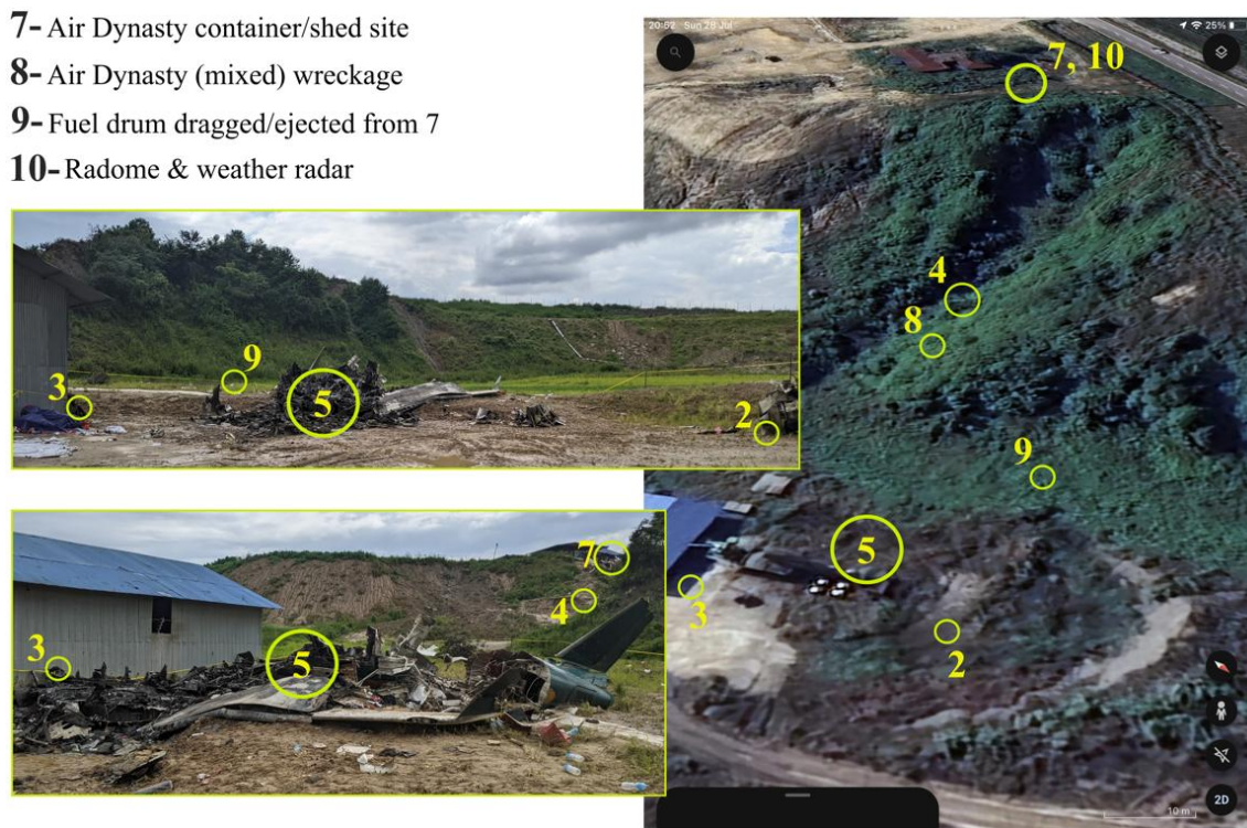
Figure 9: Overall distribution of the wreckage (see Figure 8 for markers '1' to '5')
