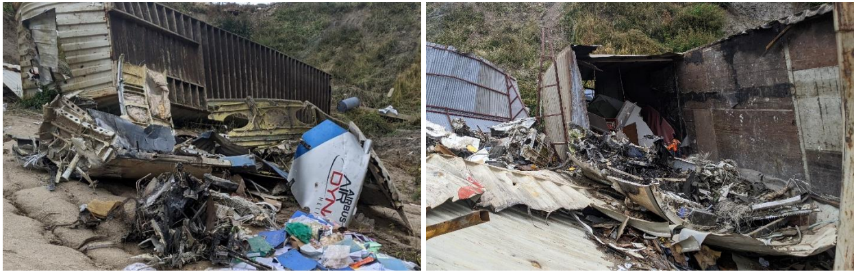
Figure 5: Accident site photos, taken on July 25, 2024, tracing the damage that occurred during the accident. [ Top-left: location of first impact by the right-wing east of runway-02 top-left; top-center-left: trail left by the right-wing as the aircraft plummeted towards the Air Dynasty shed area seen in the background; top-center-right: destroyed shed of Air Dynasty, beside the red container; top-right: crash site looking downhill of the location of the Air Dynasty shed area; bottom-left: Air dynasty container dragged down-hill by the aircraft upon impact; bottom-right: the container where the 9N-AME cockpit was stuck, showing the wreckage remaining after RFF team had taken apart the cockpit during rescue.]
