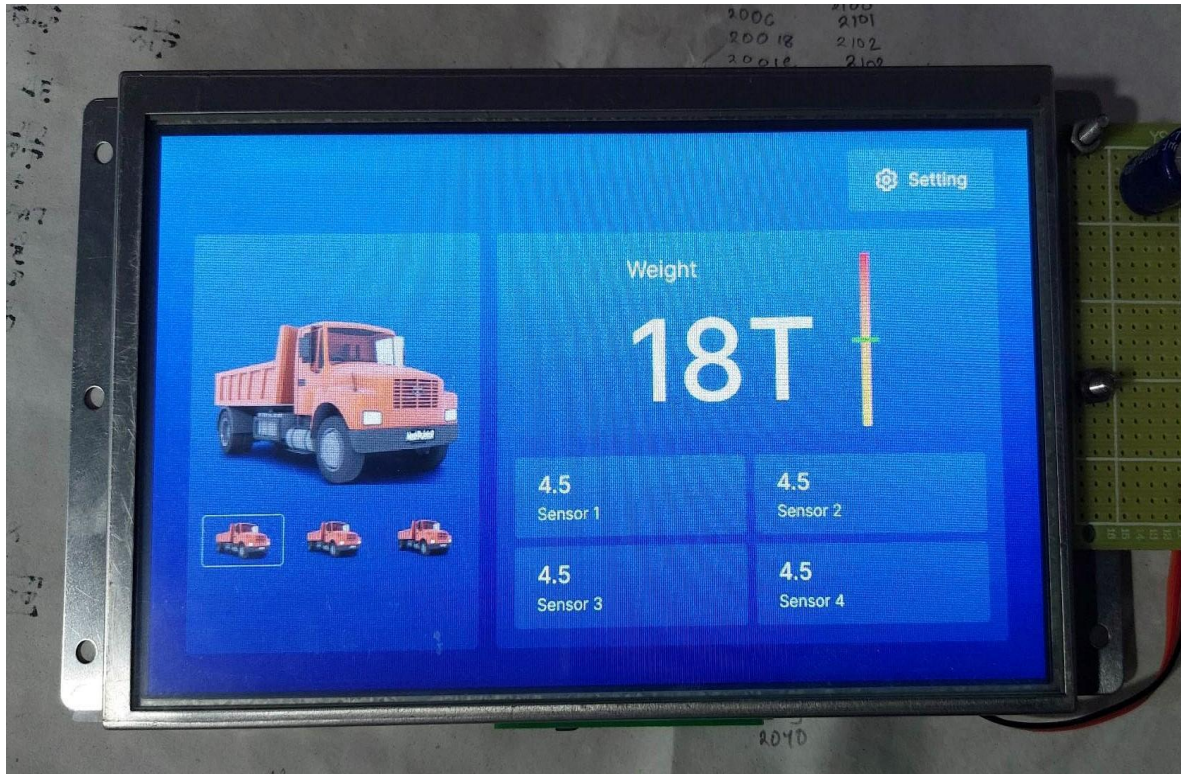
Figure 3-1: Controller showing the loading condition of the vehicle in real time
