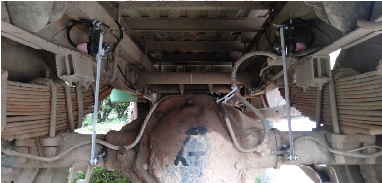
Figure 3-14: Installation of the sensors in the vehicle
