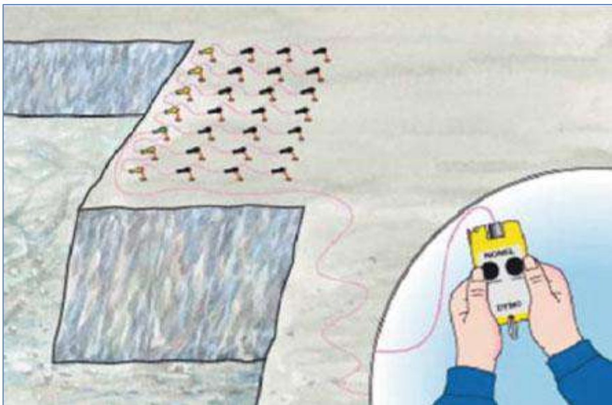
Figure 3-11 Firing a blasting round using a blasting machine (Source: Zhou, 2017)
