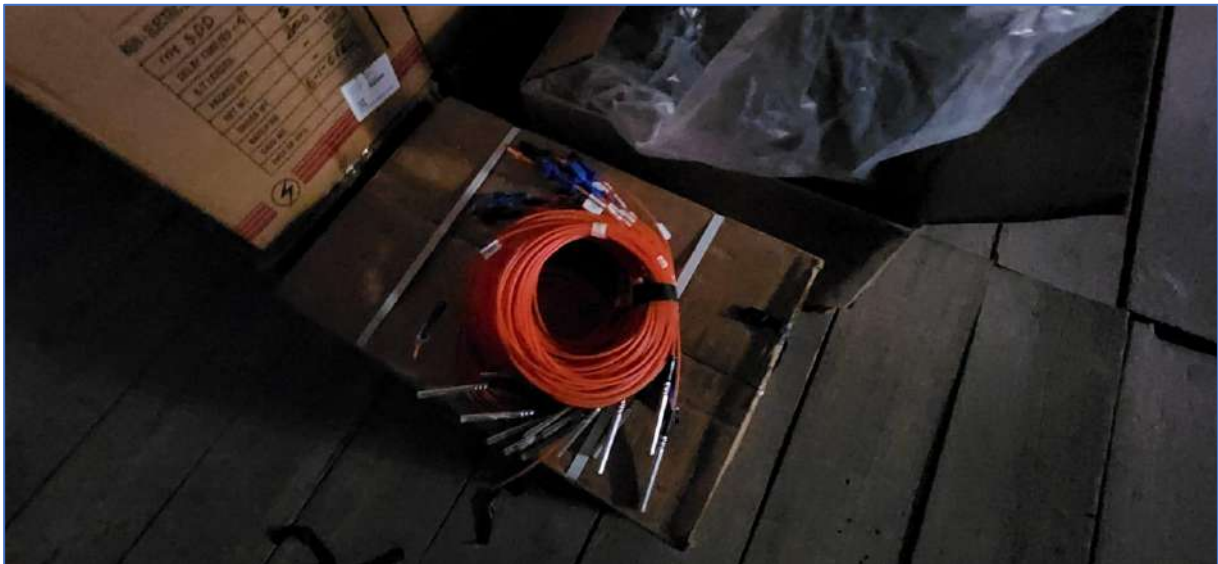
Figure 3-8 Photograph of Shock tube detonator (Non electric detonator) taken during UT-I HEP Field Visit
