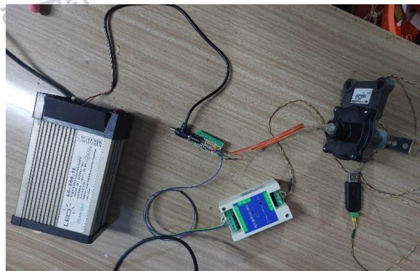
Figure 3-4: Circuit design and hardware connection of modbus
