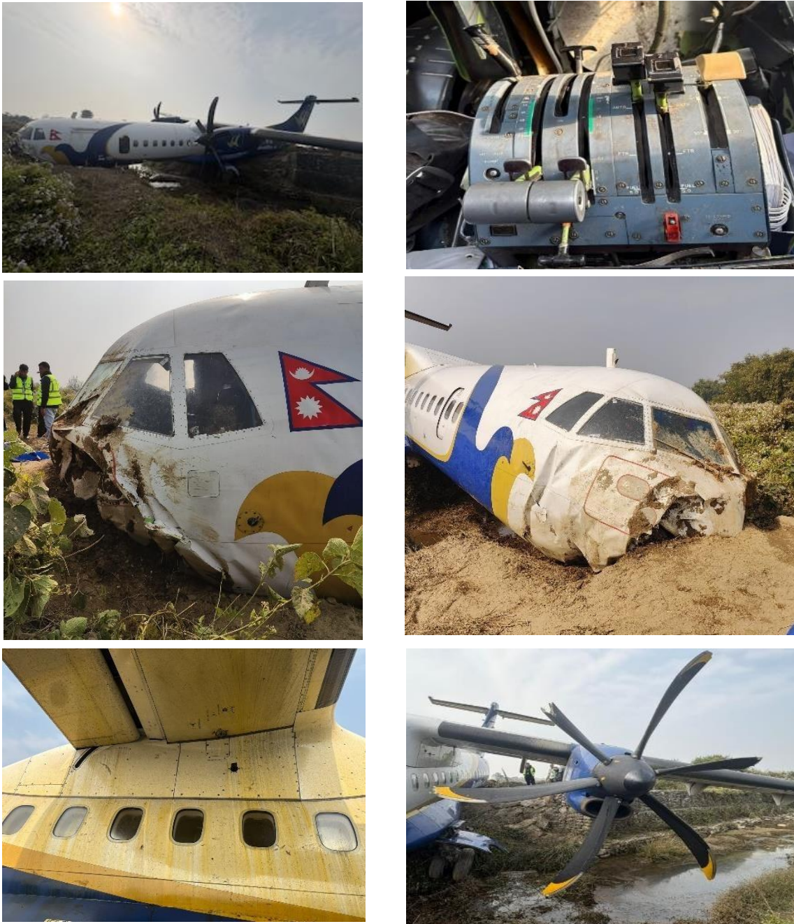
Figure 4: Wreckage of the event aircraft at VNCG, showing in situ condition of the exterior of the aircraft at the wreckage site and the position of the power (in reverse) and condition (between auto and 100% OVRD) levers
