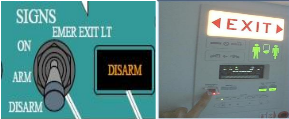
Figure 7 Emergency exit light selector in cockpit overhead panel and flight attendant panel
