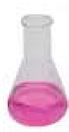
Figure 22: Colour changed during calcium determination (Purple).
