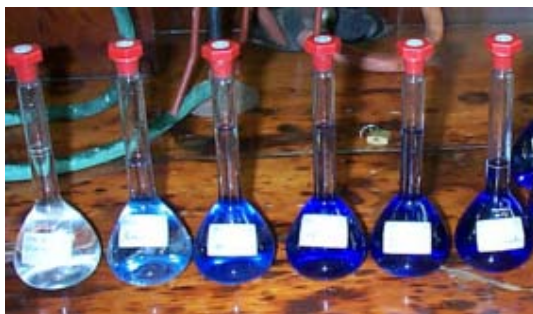
Figure 19: Showing color development during phosphorus determination.
