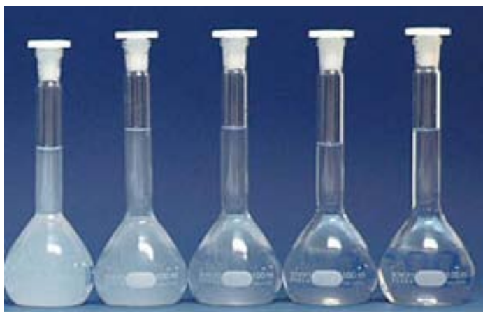
Figure 23: Color developed for sulphur determination.
