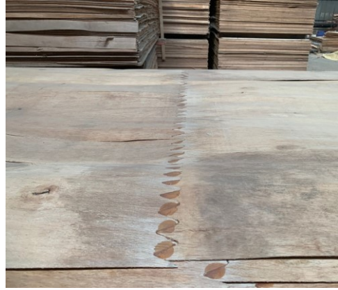
Gaining required length of veneer by joining fali
