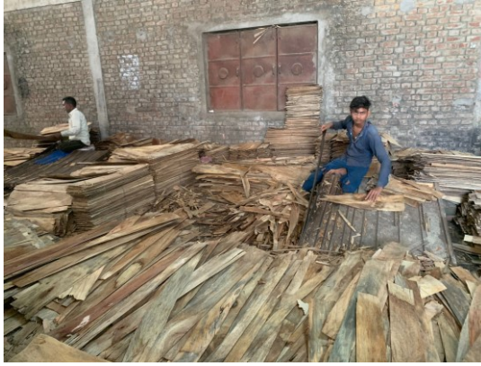
Veneer recycling to prepare fali (small sized veneer)
