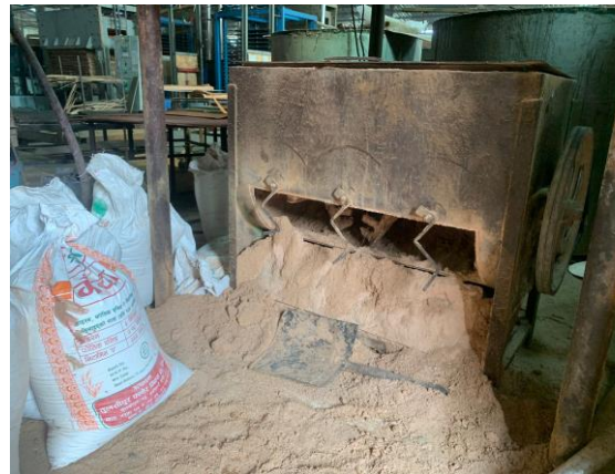
Saw dust collected from dust collector
