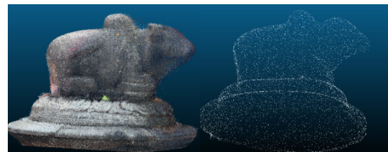
Figure 5: segmented point cloud of Case Study 1: SiteScape (Left), 3D Scanner (Right)
