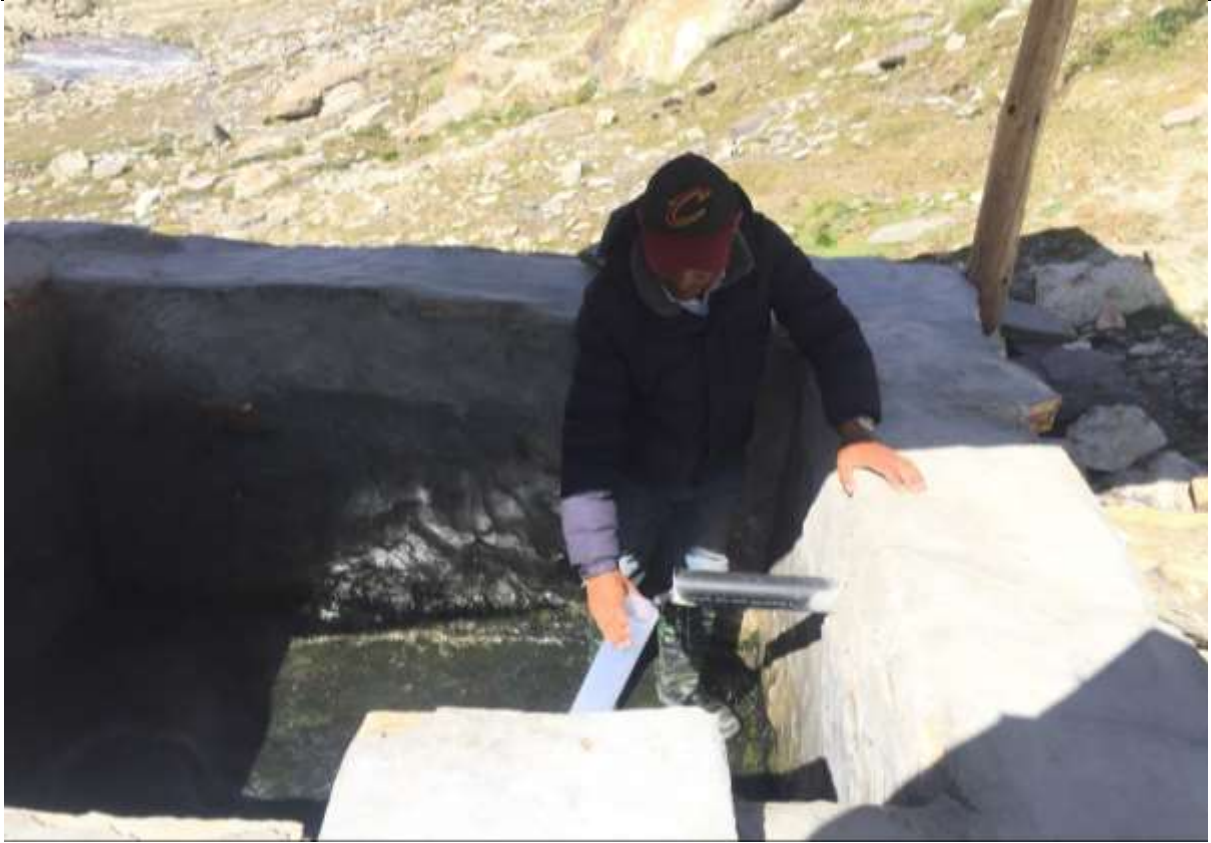
Photograph 5.58: Discharge measurement at the Takchhe Tatopani
