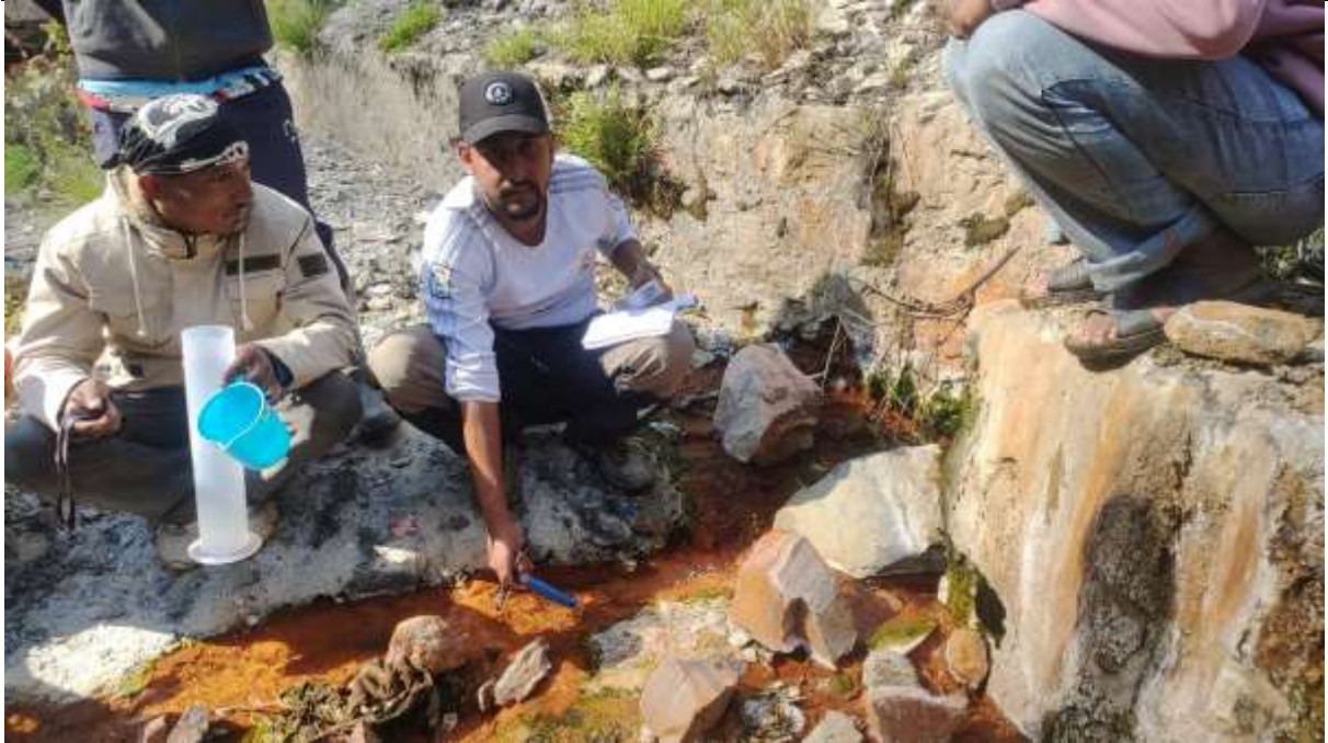
Photograph 5.62: Conductivity and pH measurement at the Darbi Tatopani
