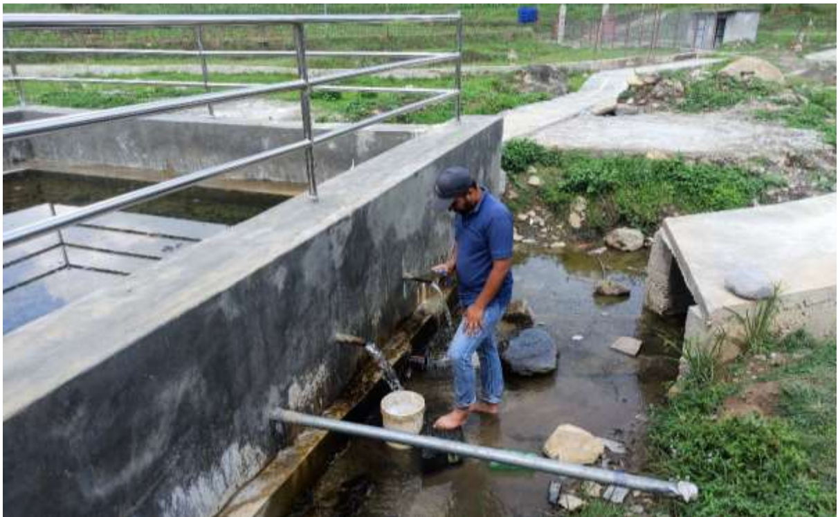
Photograph 5.11: Measurement of discharge at the Bhulbhule Khar Tatopani
