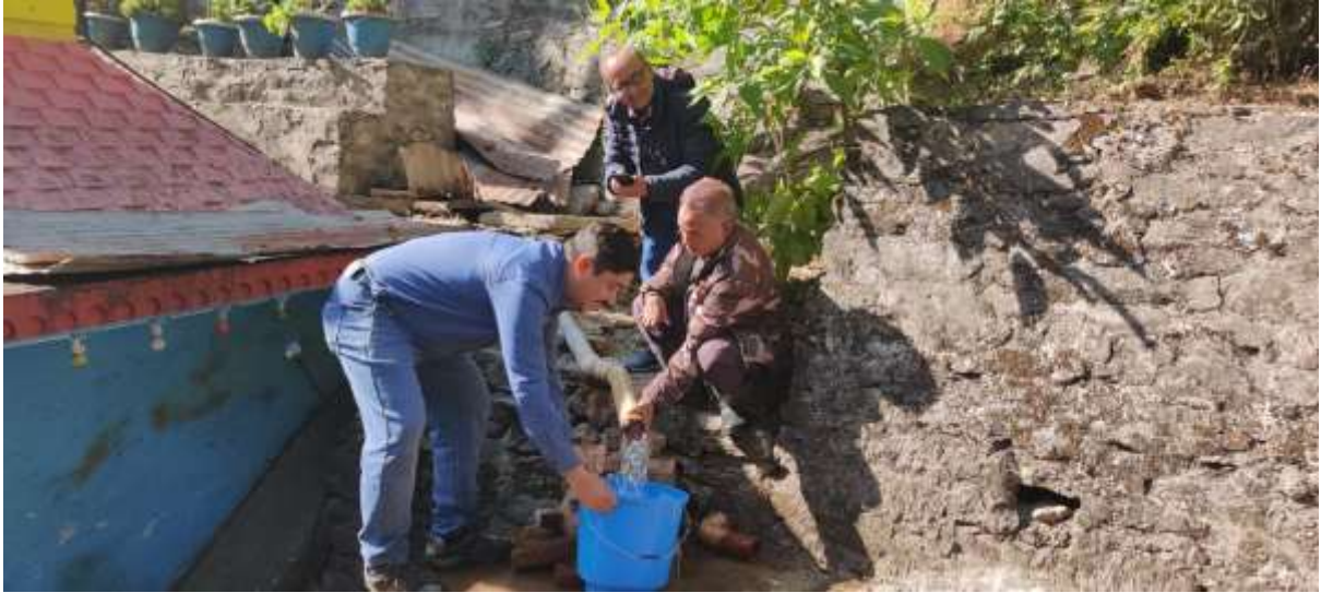
Photograph 5.2: Discharge measurement at the Tatopani Dhara
