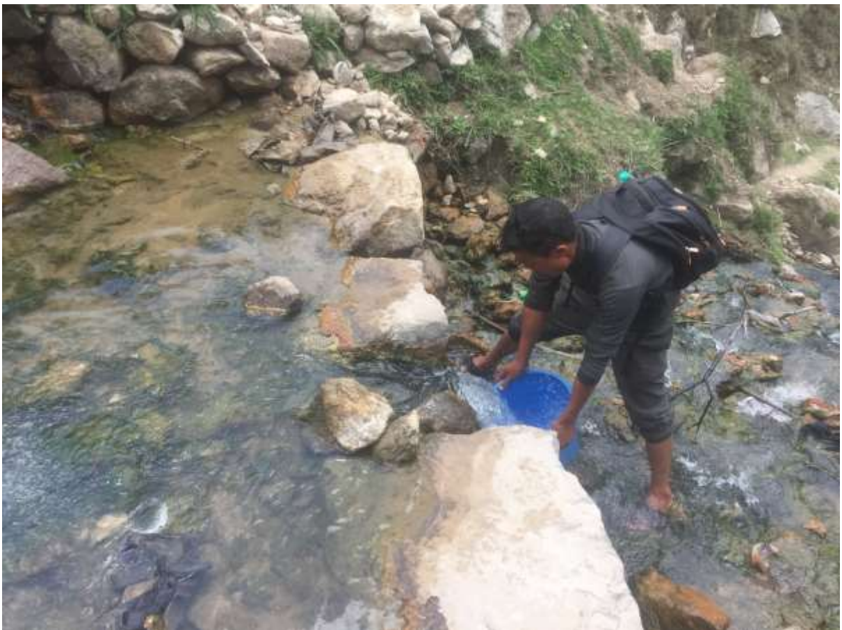
Photograph 5.56: Discharge measurement at the Kermi Tatopani
