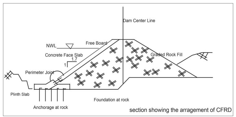
the pressure exerted by the concrete slab and the water pressure when the reservoir is full of water. This capacity of the rock embankment is tested by measuring the modulus of deformation and should be within the range of 50 Mpa to 100 Mpa.
