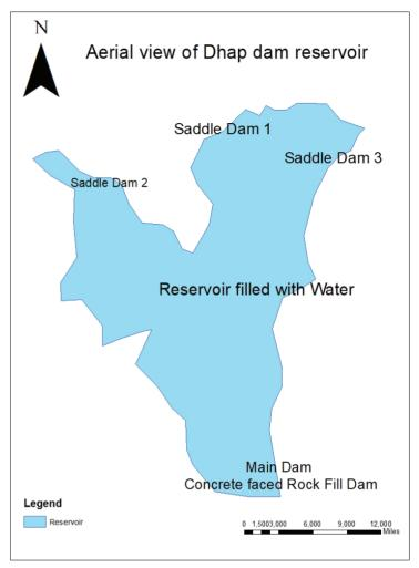
The Dhap dam with maximum height of 24 meter, the anticipated settlement is 24 centimeter. The provided free board, which is the allowance for settlement of crest due to earthquake, provided is 3 meter above the normal reservoir level. This shows that even in the earthquake having peak horizontal ground acceleration up to 0.82, the water from the dam will not spill over the crest thus keeping the dam body intact even with the shock generated by ground motion.
