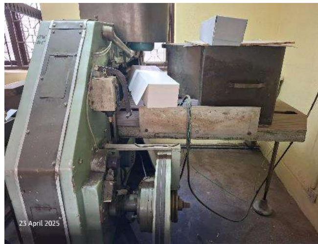
Safety guard removed from machine.
