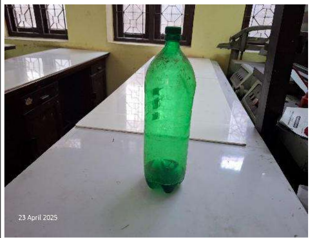
Chemical stored in water bottle without labelling.
