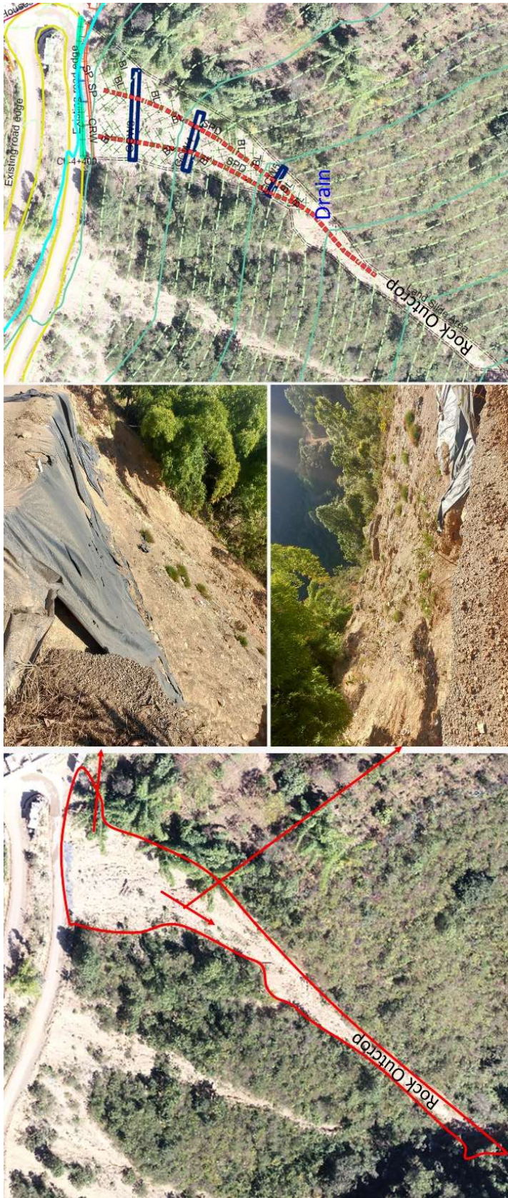
Figure 7.6: Shallow seated landslide: Site photographs, landslide map and proposed mitigation measures
