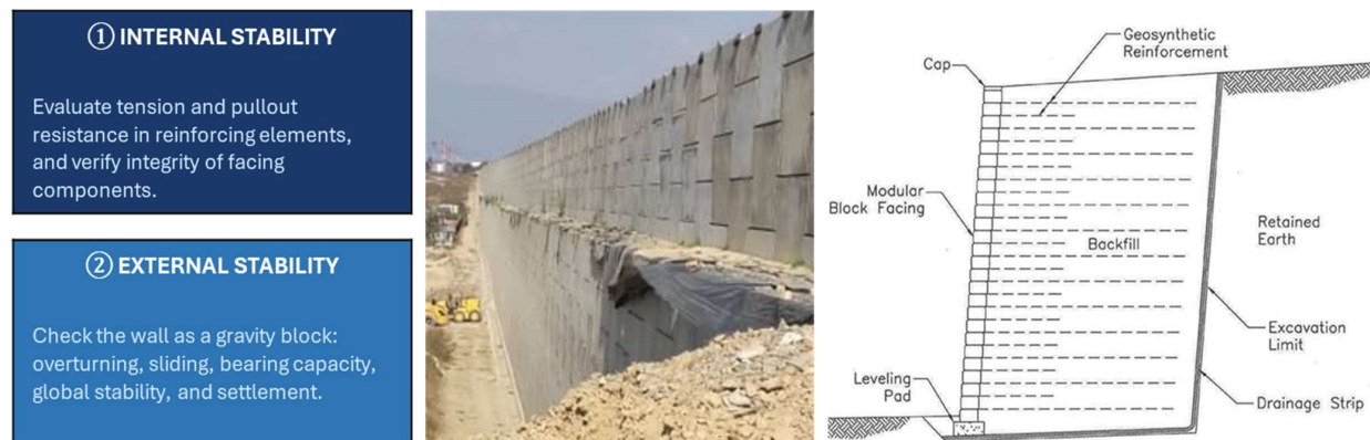
Figure 4.12: Mechanically stabilized earth wall
