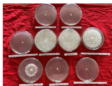
Figure 2. Poisoned food technique with fungicides at 25 ppm
