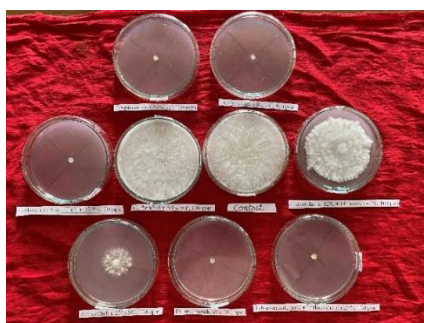
Figure 3. Poisoned food technique with fungicides at 100 ppm
