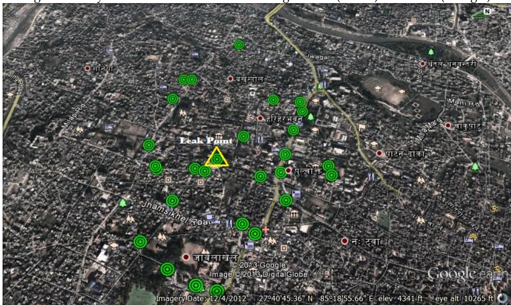
Fig. 11. Survey around Pulchowk area indicating no-leak (circles) and a leak (triangle).
