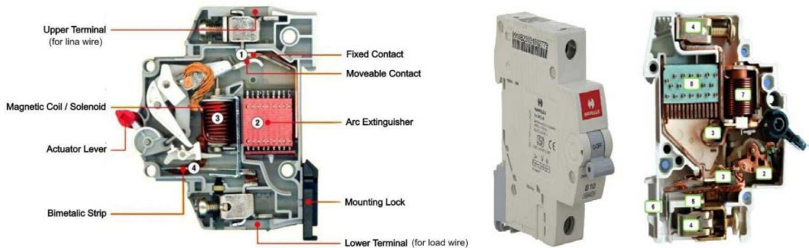
Figure 4.5: Construction of MCB
