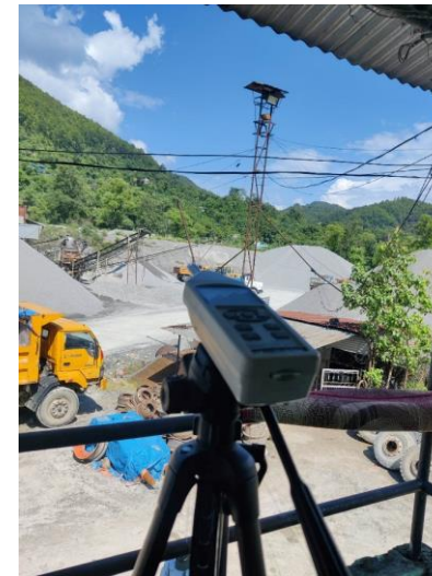
Pic 16: Noise Level monitoring at N3 site
