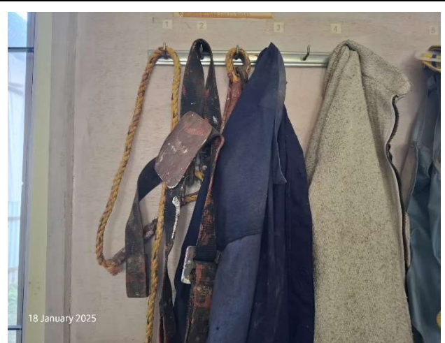
Safety harness was contaminated.
