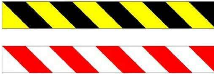
Figure 4-1 Signage for Obstacles and Dangerous Location
