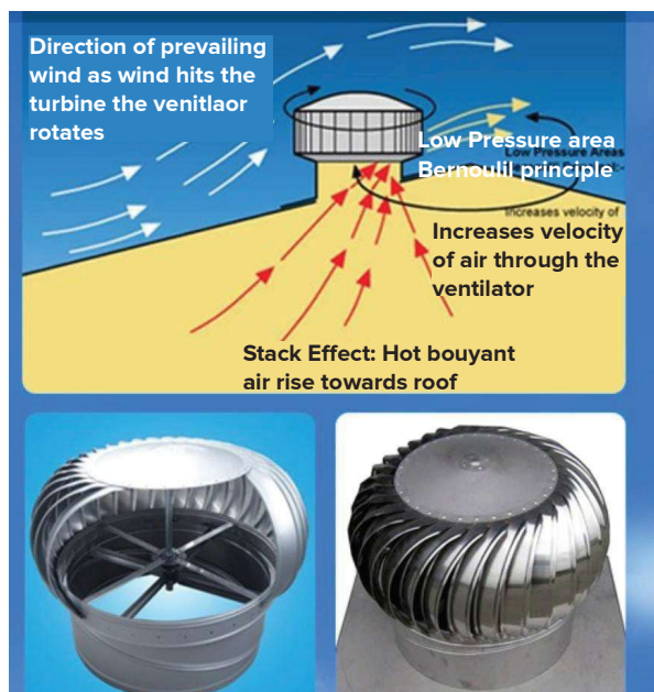
Figure 71: Turbine roof Ventilator
